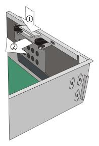
Lift up the drive and remove it. Loosen the connecting cables.
