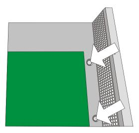
Carefully tilt the hard disk carrier into the orginally position. Make sure that the drive holder will not pinsh cables. The metal tangs snap in place.
